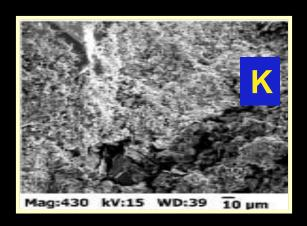
Kaolinite (K)"books" filling center of pores while chlorite coats quartz grains.
