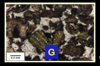
Bioclast filled with intraparticle glauconite (G).
