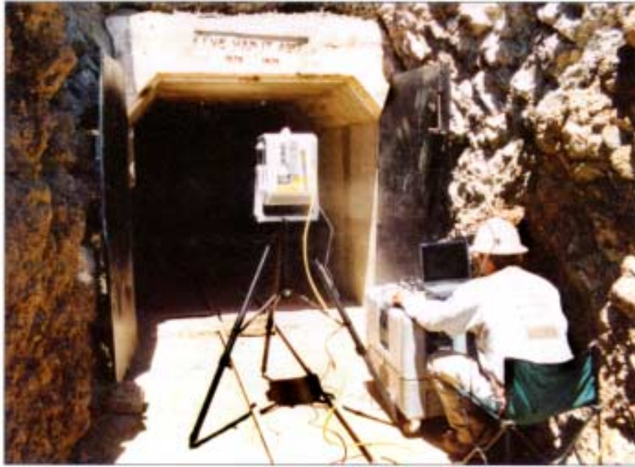
Figure 1. The laser scanner is laptop-controlled and reasonably portable. Here, it is set up for mapping fractures in the San Xavier Mine, south of Tucson, Arizona.
