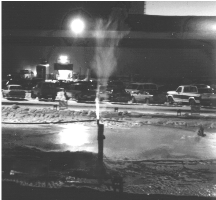
FIGURE 2 - Gas flaring from a 30m test hole in pulp mill parking lot 20km north of the Town of Peace River.
