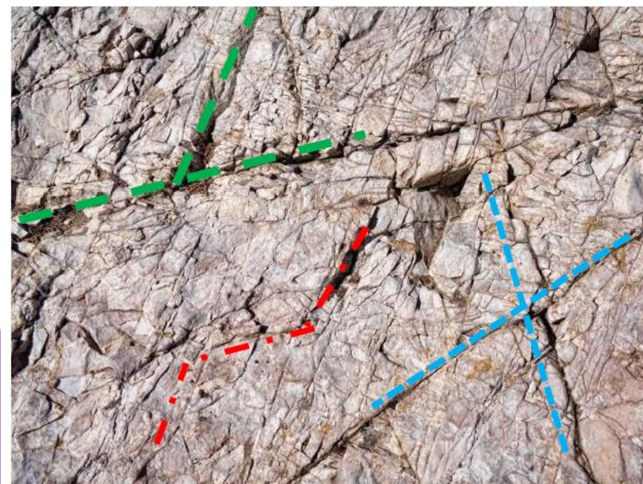
Fig 1. The prevalent naturally occurring fractures in a rock outcrop are showcased by their distinctive colors: X-shaped fractures are represented in blue, Z fractures in red, and Y fractures in green. Ifrene et al (2023)
