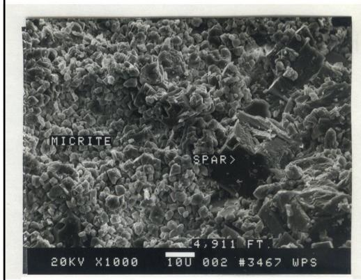
1000X - 4,911' - High magnification reveals the difference between calcite spar infill and micritic calcite. Note the intergranular microporosity within the micrite. This type of porosity could generate matrix flow.
