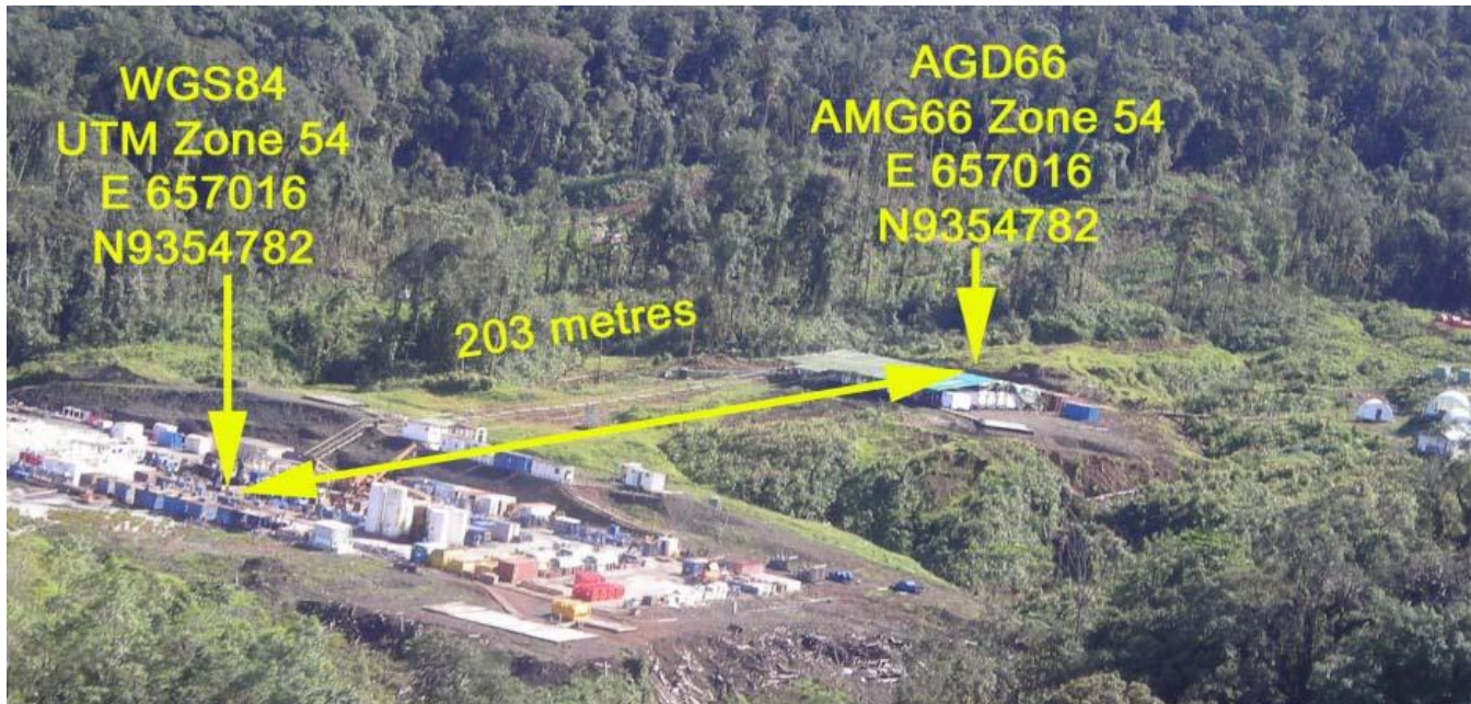
Figure 1. 200+ m difference between WGS84 and AGD66 in PNG.
