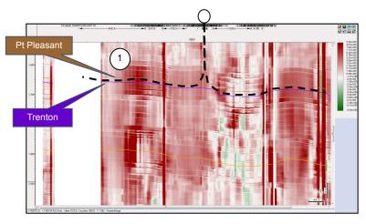
Structural sags (green) may point to karsting/collapse, but not necessarily. Can Paradise discriminate the altered sags vs the non-altered ones?
