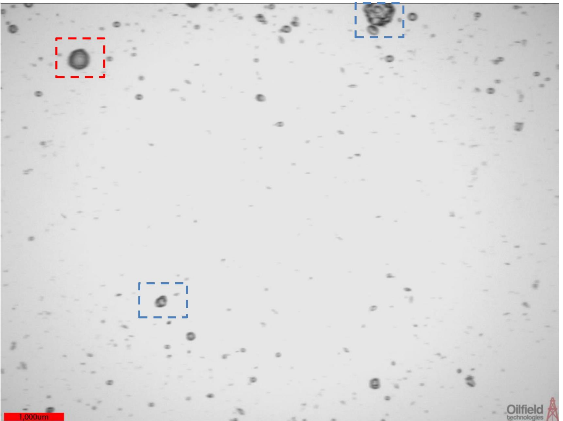
Figure 4. Water, hydrate, and gas bubble flow. Beginning of hydrate formation.
