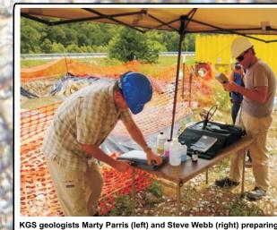
to collect a formation water sample from the lower Copper Ridgi step-rate test interval prior to the test.
