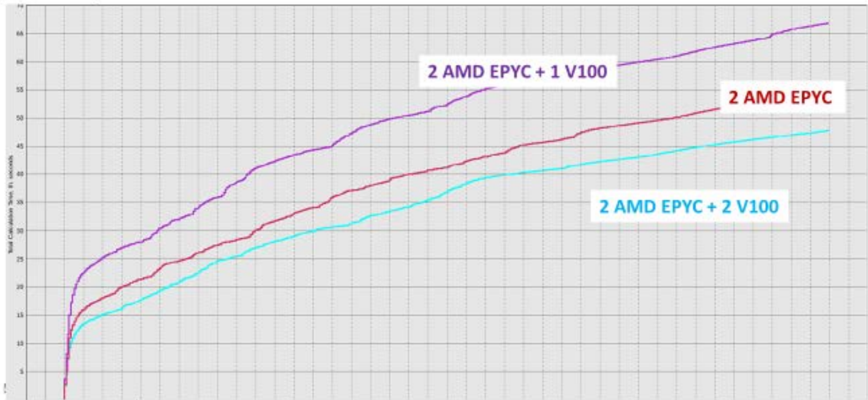
Figure 7. 18 million active blocks, dual porosity black oil model. 10 wells with multistage fractures and LGR's, 50 years production forecast. Total calculation time.
