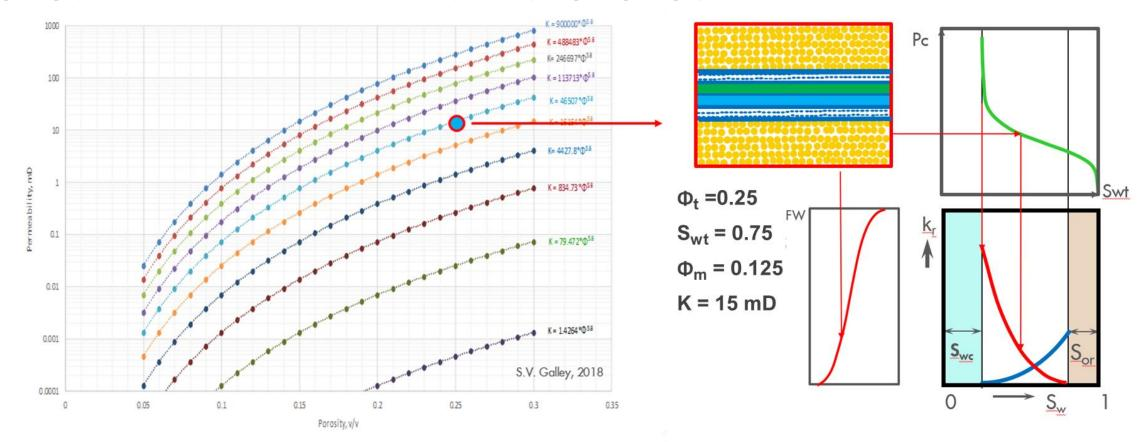
In this case irreducible water occupies 50% of total porosity which is located sufficiently high above free water level (FWL), so amount of movable water is negligible. If reservoir engineer uses standard Brooks – Corey equation, connate water saturation will be about 18% and rock will produce 50% water cut. Obviously such high water cut contradicts production data, which has about 4% water cut. So what reservoir engineer do?
