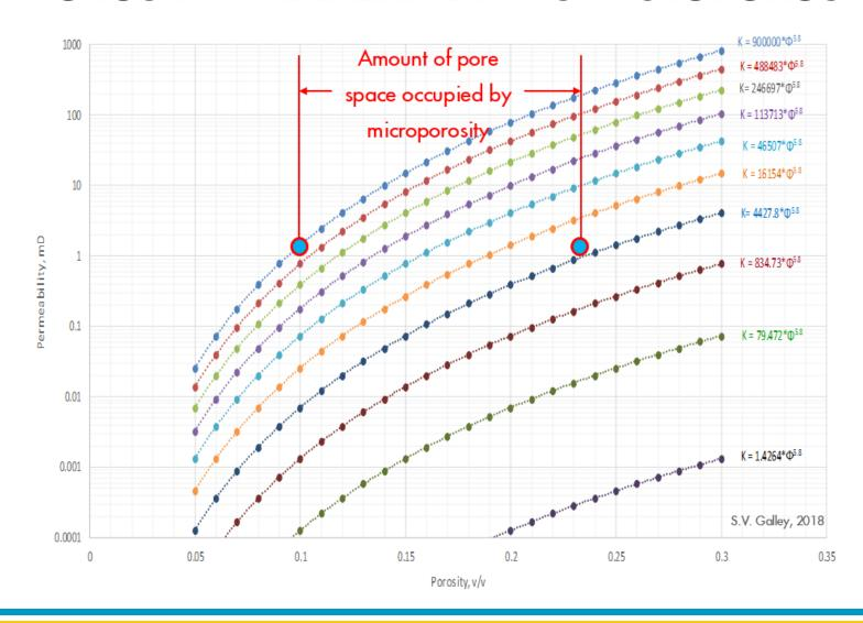
Two points with same permeability have different porosity, which means that difference between these two is amount of microporosity, holding all other variables constant. This microporosity is added on top of connate water calculated by standard Brooks – Corey saturation height model.
