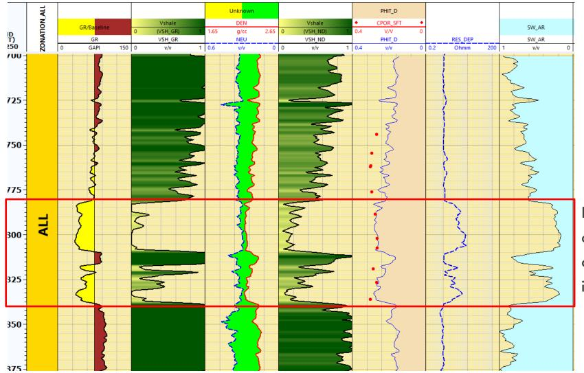
Interval for completion, based on conventional interpretation results.
