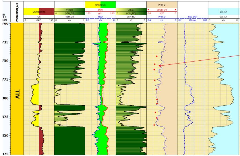
Porosities do not match the core porosities, unless thin bed analysis module LowReP is utilized.
