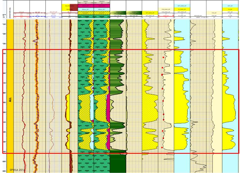
Interval for completion, based on thin bed analysis interpretation results.
