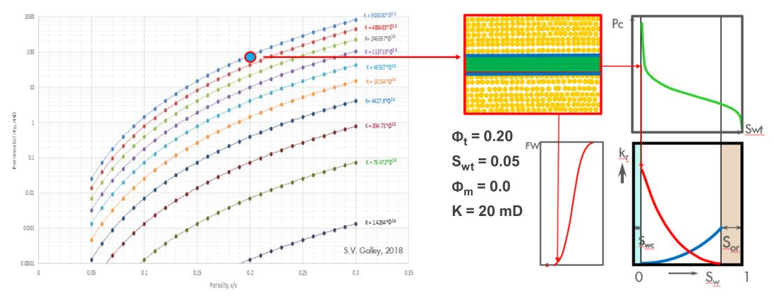
Clean sandstone end member has irreducible water saturation, defined by cap pressure curve, which is water covering grain surfaces (water wet rock).
