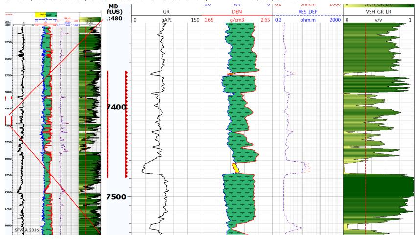
This is second to the best well in Gulf of Mexico. Mostly thin beds with high reservoir properties. If standard cut-off  $V_{shale} = 0.3$  would be used, this well would be never perforated.
