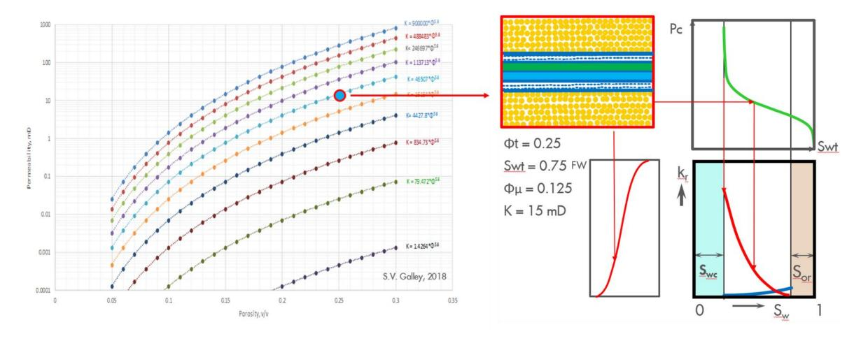
Reservoir engineer increases water Corey exponent and suppress water flow. However, water relative permeability is rather unphysical, it could be possible only when water viscosity is significantly higher than oil viscosity.
