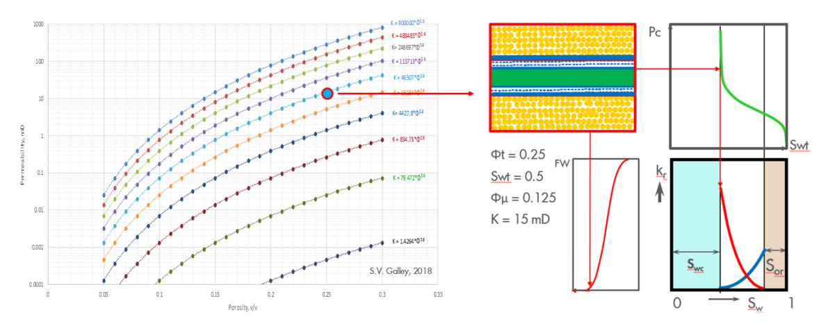
Relative permeability end points are shifted to match position of connate water saturation point. Corey oil and water exponents matching core derived value and production is water free, assuming this interval is sufficiently high above FWL.
