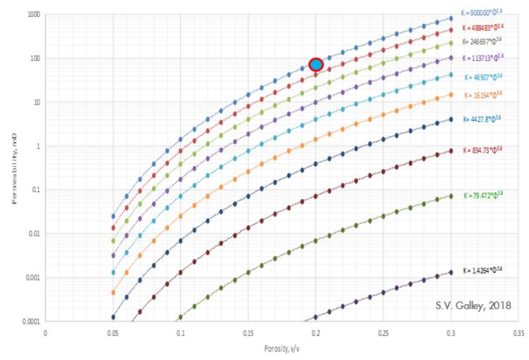
Position of porosity and permeability point on this chart is also controlled by amount of microporosity.
