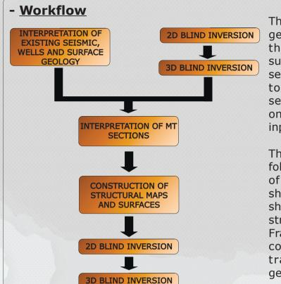
The interpretation process began with the generation of a geological model based on the 2D seismic information, the geological map, dip and azimuth data from the surface, and the well data. Secondly, the MT - Resistivity sections were added to the interpreted sections in order to compare both responses. Then, the geo-electric sections and seismic sections were correlated. Finally, once the information was confirmed it was used as the input for the constrained inversión.
