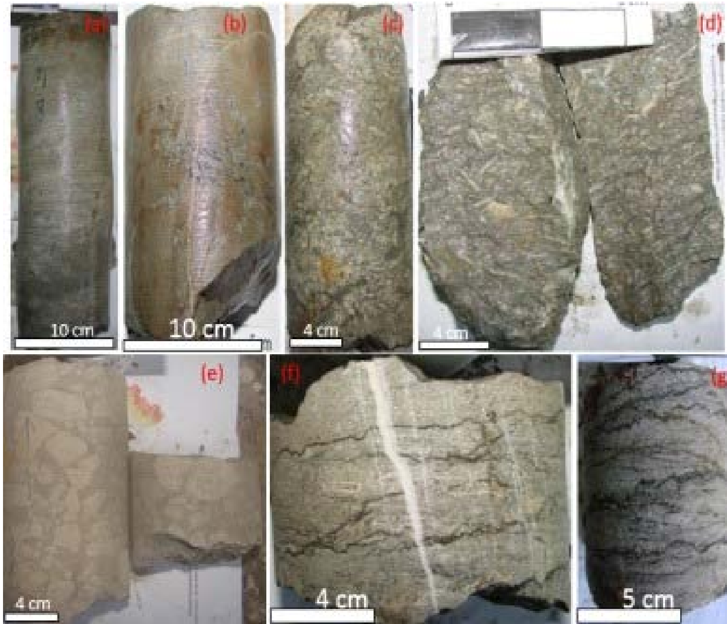
Figure 13. (a and b) Buff to dirty white micritic mudstone to wackestone (TST part), (c and d) Wackestone to packstone in the HST part, (e) Intraclastic limestone with rounded limestone fragments, (f and g) Low angle stylolitic laminae observed within Sylhet Formation.
