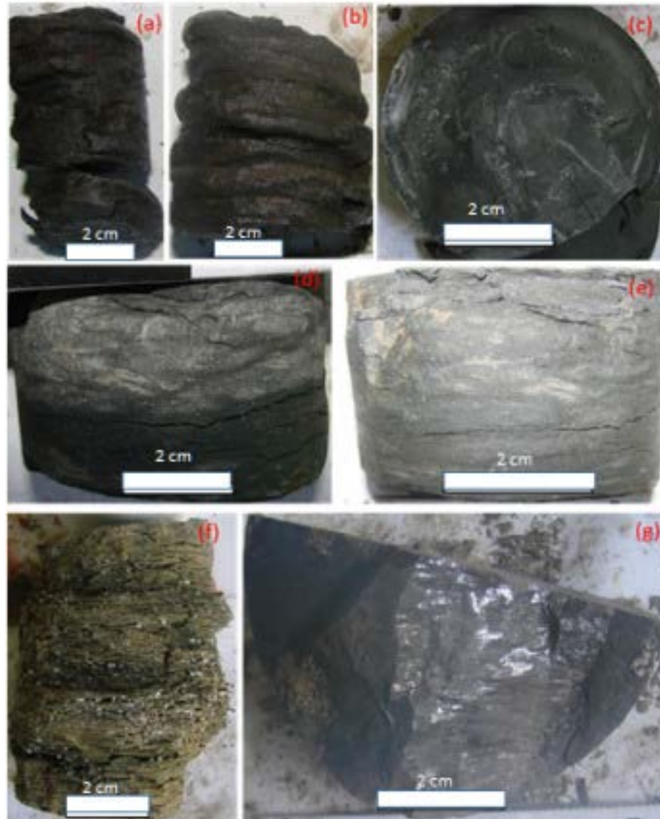
Figure 4. (a and b) Grey to reddish, hard, moderately to poorly fissile silty shale (facies 2a), (c) Carbonaceous shale with devoid of any tidal imprints (facies 2a), (d) Shale with sandstone/siltstone lenses (facies 2b), (e) Greenish to grey shale (facies 3a), (f) Occurrences of striated and polished slickensides within facies 3a.
