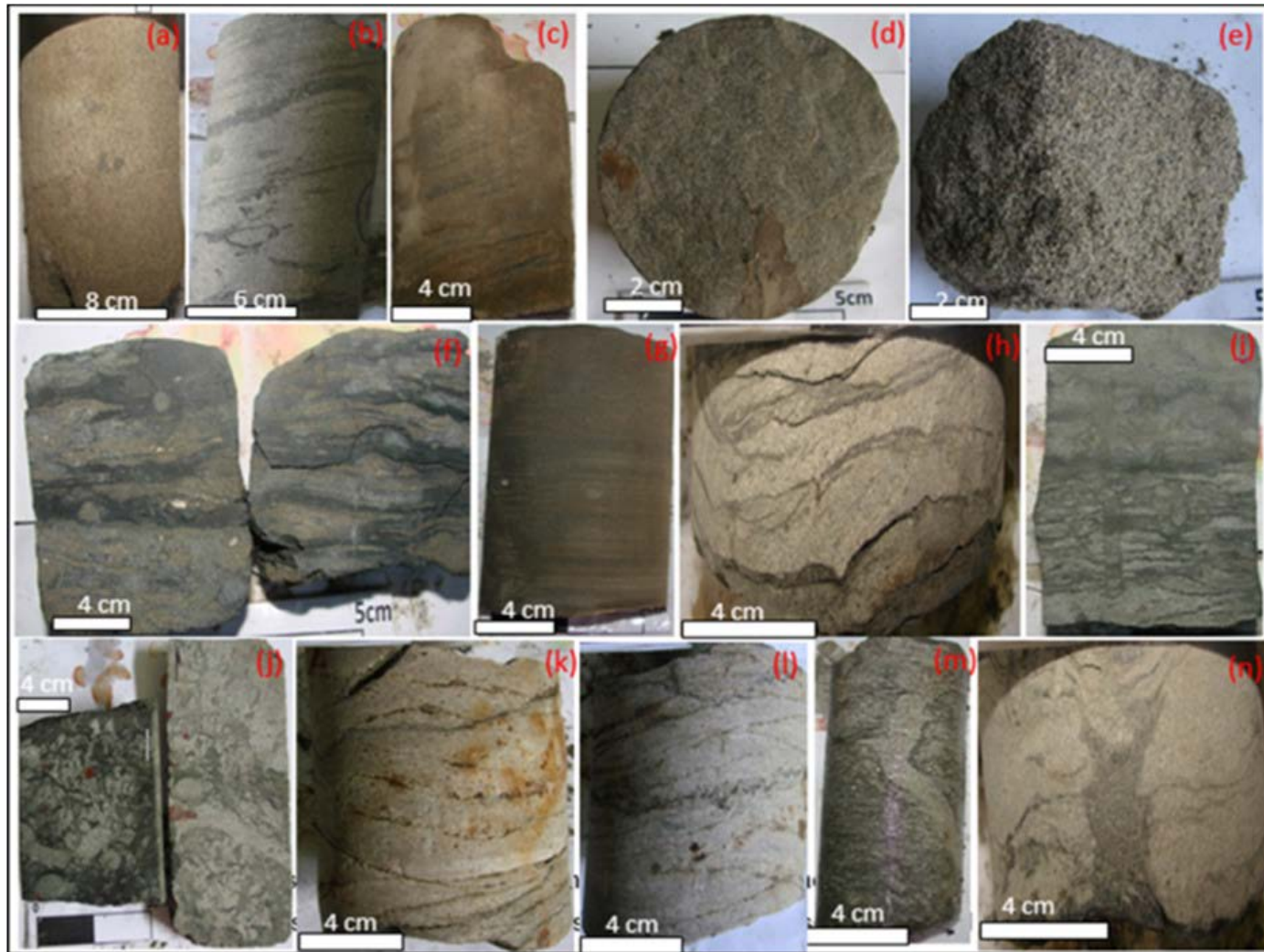
Figure 3. (a) Massive argillaceous sandstone, often fining up (facies 1b). (b and c) Cross-stratified fining-upward sandstone representing facies 1c, (d and e) Coarse-grained well-sorted sandstone characterised by facies 1d, (f) Sandstone-shale heterolith (facies 1e), note sharp change in lithology due to tidal fluctuations, (g) Rhythmic alternations of sandstone-shale laminae, note occurrences of double mud drapes, (h) Penecontemporaneously deformed mud laminae, (i) Heterolithic facies gradually changes into shale, note in the lower part bidirectional ripple laminations and thin flaser beds. (j) Profusely bioturbated heterolithic facies, (k and l) Wavy, ripple laminated sandstone (facies 1c), note bundle wise up-building and draping-offshooting wave ripple lamination, (m) Vertical skolithos burrows within bioturbated heterolithic facies (facies 3D), (n) Mud injection as a result of penecontemporaneous deformations.
