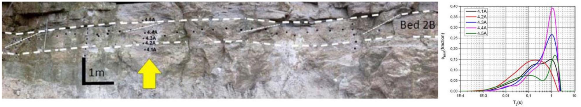
Figure 2. Pore distribution from a short NMR profile in the Morro do Chaves Fm (from De Luna et al., 2016).
