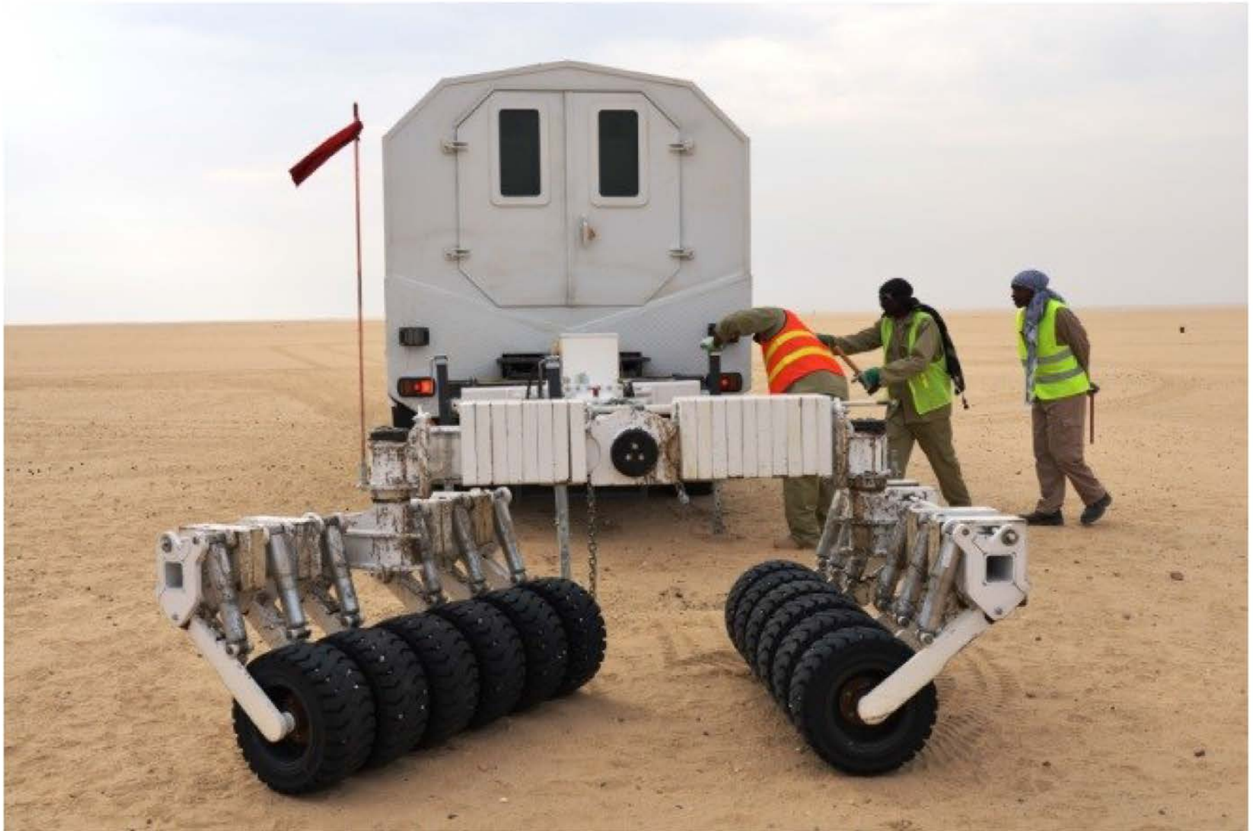
Figure 10. Armored Vehicle deployed for mine clearance.
