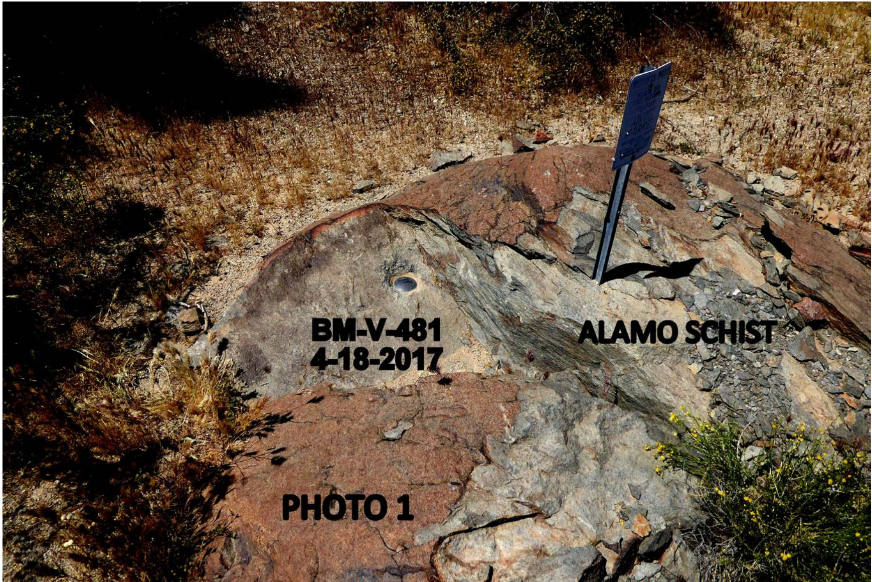
Figure 3. National Geodetic Survey Bench Mark BM-V-481 (1981) is cemented into a large boulder of Alamo Schist on the west side of Alamo Road ( Figure 2 ).
