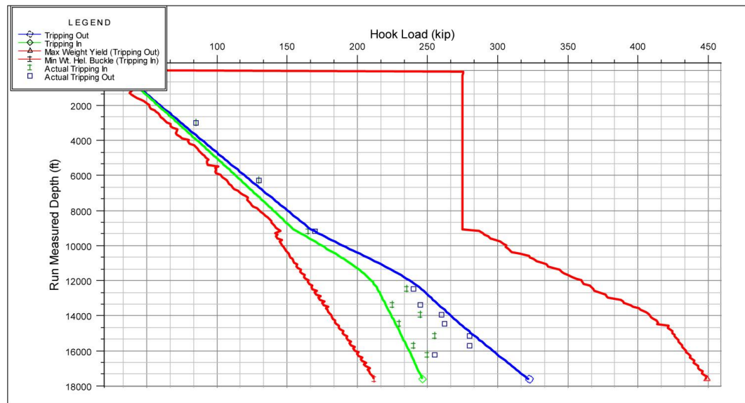
Figure 2. Hookload graph of reaming trip with input of actual loads.
