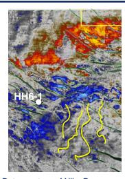
Data courtesy of Niko Resources: Flattened seismic volume on the 'HH6-1 Gas' pick and then took a couple of time slices. Reds and yellows are troughs, blues are peaks.
