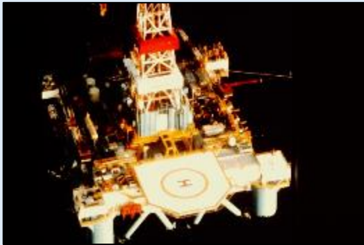
Semi-submersible drilling rig on location offshore California
