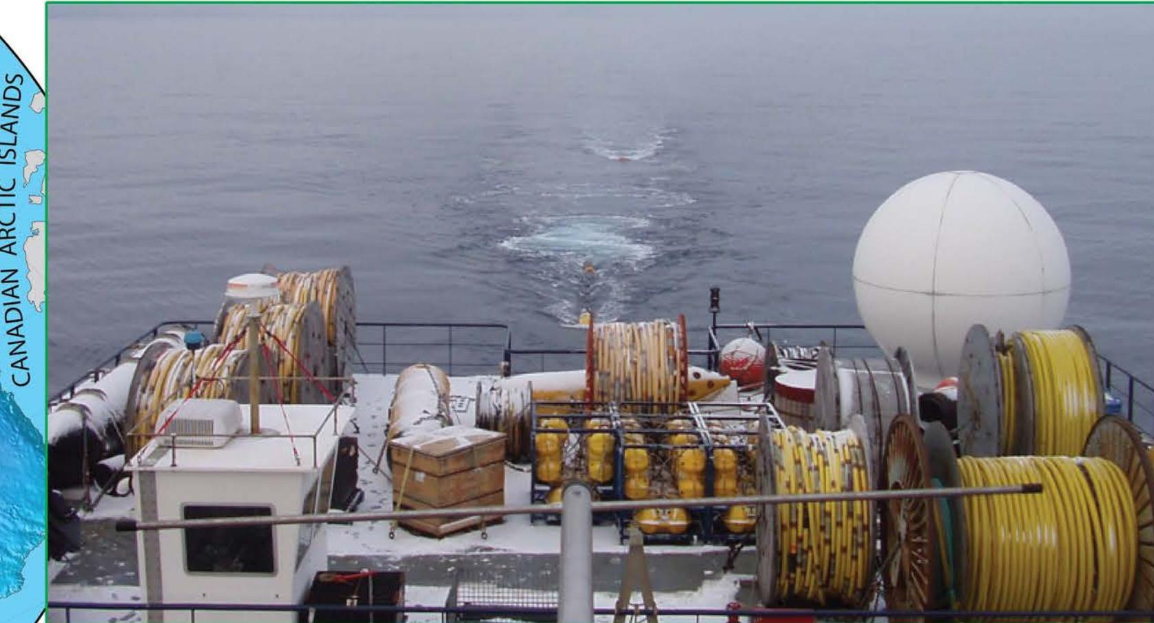
Acquisition of multi-channel seismic reflection profiles in 2011 by the *R/V Marcus G. Langseth* across the transition from the Chukchi Shelf to Borderland
