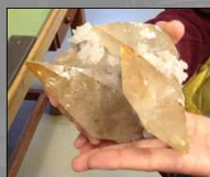
Figure 3: Calcite (common gangue mineral associated with MVT ores) containing hydrocarbon fluid inclusions (Elmwood Mine, Central Tennessee District).
