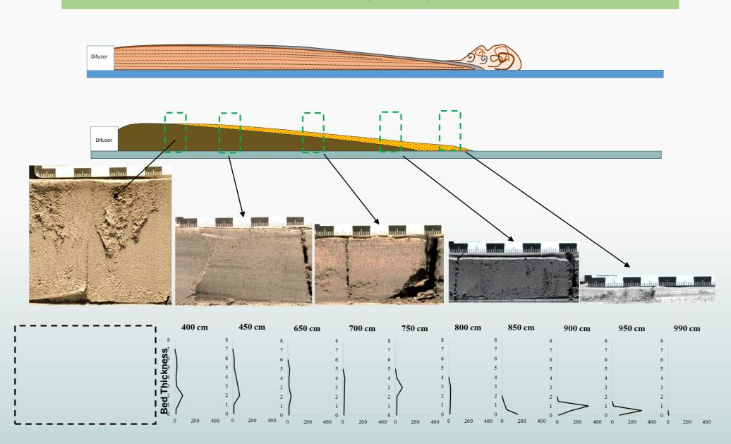
Newtonian Low-Density Currents like flow develops high velocity however low efficiency (non homogeneity).
