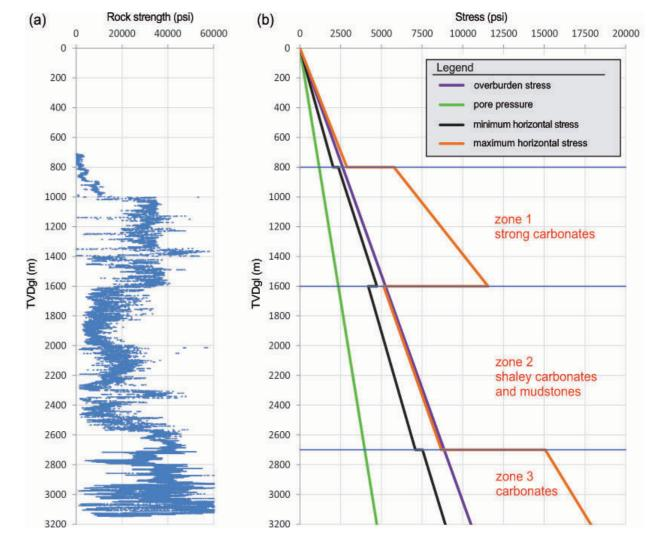
This in situ stress profile was constructed by:
