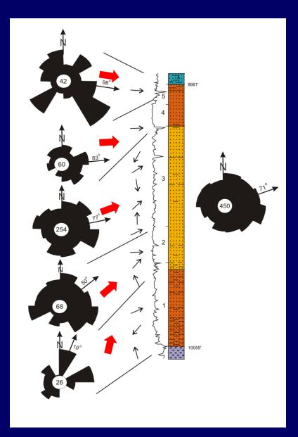
Rose diagrams based on depth calibrated FMS imaging data of the Sarir Sandstone cross-bedding inclination azimuth
