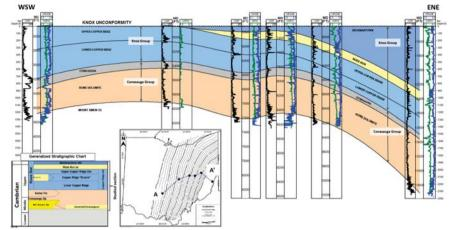
WSW to ENE (A-A') Cross Section of the Study Area Showing Change in Sediment Thickness in an Eastward Direction (Note: Knox Unconformity surface was used as datum)
