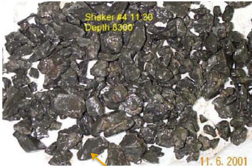
Blocky Cavings – Evidence of Fractures
