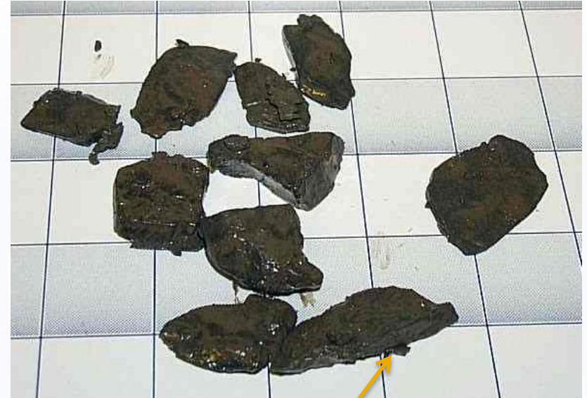
Platy Cavings – Evidence of Weak Bedding
