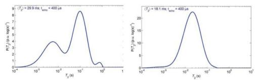
**Figure 2:** Two examples of T2 distributions for plug in the study, left, a clearly bimodal plug, right a unimodal one.
