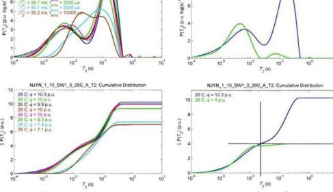
Figure 3: Changes to the T2 distribution shape and total detected porosity as a function of echo spacing are used to estimate internal gradients. In this case, virtually no changes for echo up to 1000 µs suggest negligible internal gradients.
