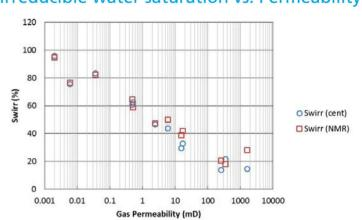
**Figure 10:** Relationship between permeability and irreducible water saturation after spinning in the centrifuge. Saturation from NMR (water filled porosity) and from produced fluid match very well for lower permeability samples while the scatter increases a bit for lower irreducible saturations (higher permeability samples).
