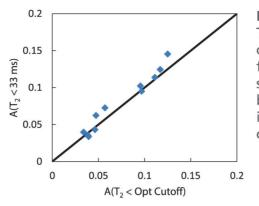
Figure 5: Comparison of the NMR T2 signal below 33 ms (standard cutoff) and the optimised cutoff for each sample. The consistency suggests that the cutoff-based bound fluid model is robust even in the presence of variations in the cutoff.
