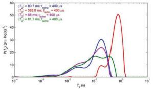
The extremely high relaxivity required to obtain a good match can be indication that the isotropic sink model approach adopted in the simulation is too simplistic and requires the implementation of a more complex dynamics.
