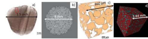
**Figure 12:** a) An optical image of a standard 1.5 inch plug and location of the mini plug extraction (8 mm diameter), b) an X-ray image of the mini plug, c) a lower resolution numerical model (pixel size 2.15  $\mu$ m), and d) a higher resolution numerical model (pixel)
