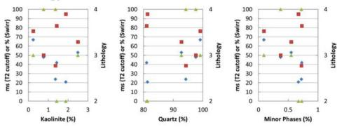
Figure 11: Relationship between chemical composition from Qemscan (left to right, kaolinite, quartz and minor phases) and measured parameters. The "lithology" is a dimensionless parameter extracted from MICP curves by inspection, and is an indication of the production quality of the rock. Note that none of the parameters correlate with the chemical composition.
