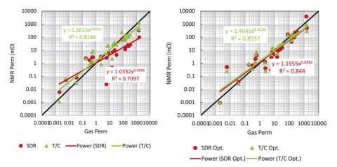
**Figure 8:** NMR derived permeabilities vs. gas permeability (both SDR and Timur-Coates). Left: Using standard parameters. Right: Using optimised parameters (see table).
