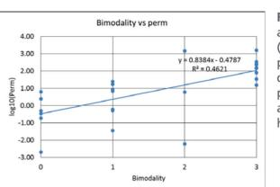
Figure 9: Relationship between an estimation of bimodality (from eye inspection) and permeability. Although highly qualitative and subjective this plot shows the plugs showing a higher degree of bimodality have higher permeability
