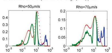
**Figure 7:** Examples for two different plugs. Left: a case where two peaks are clearly identifiable but different relaxivity is required to match each of them. The right panel shows two peaks that match using the same relaxivity.
