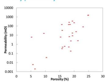
Figure 1: Permeability versus porosity for the plug studies.
