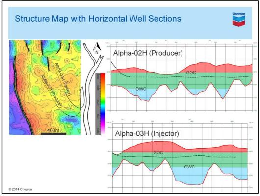
Presenter's notes: The map on the left is a structure map on top of the sand based on well control and seismic and shows the two horizontal wells Alpha-02H and Alpha-03H which were drilled as platform infill wells in 2012
