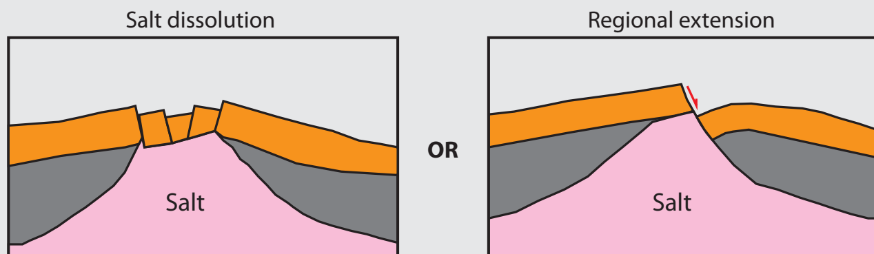
Figure 1. Previous proposed models for diapir fall / salt collapse structure (after Ge et al., 1996)
