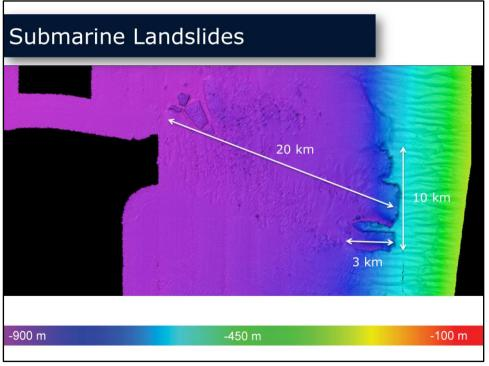
Presenter's notes: Another factor controlling slope facies is instability. Submarine landslides of this extent are spectacular. Indicators for creeping and slumping can be seen all along the slope. Gullies all along the slope from very north tol very south show a spectacularly organized trend of equally spacing of 350 m.
