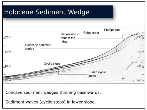
Presenter's notes: This is a subbottom profile across the slope. In general, during highstands, the platform produces sediment, and currents transport the fines downslope where they accumulate in a so-called sediment wedge. The strong reflectors delimit the wedge and are lithified lowstand surfaces. Behind the plunge pool, on top of the wedge there is a coarse-grained ridge.
