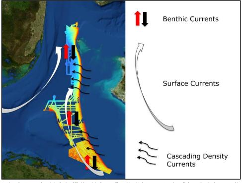
Presenter's notes: Besides two main surface currents, through the Straits of Florida and the Santaren Channel, benthic bottom currents and so-called cascading density currents, driven through water-salinity gradient in summer and water-temperature gradient in winter, influence the sediment patterns and distribution along the slope
