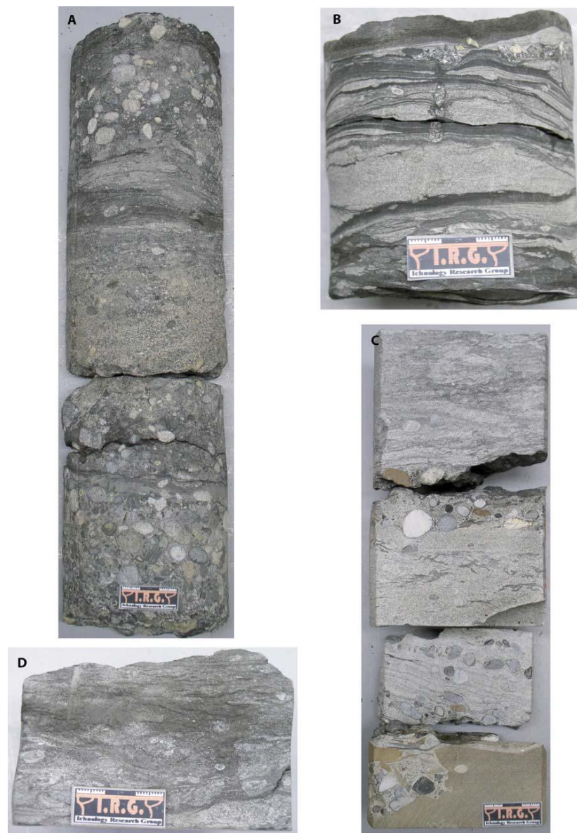
Figure 3. Expressions of the uppermost transgressive surface of erosion demarcating the top of the Viking Formation. (A) Two pebble horizons in the lag above the TSE in well 08-01-036-22W4. (B) Skolithos infilled with coarse sand lag highlighting the Glossifungites surface at the TSE in well 02-04-037-19W4. (C) Sideritized firmground overlain by a pebble rich deposit in well 16-11-031-24W4. (D) Apparent gradational contact from Viking deposits to Westgate Shales in well 02/07-22-038-20W4.
