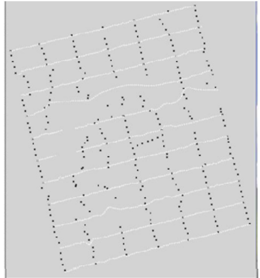
Figure 3. Moose Mountain 3-D survey layout. Dark circles are shotpoints and white lines are the receiver lines.
