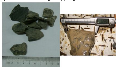
Figure 1: Typical recovered shale cavings from Field A in Bohai Bay, China (from Wu and Tan 2010)
