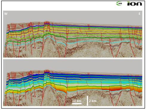
Presenter's notes: At the top you can see the seismic line along with our inputs, meaning previously interpreted horizons and faults. In the image below you can see the same line with the auto-tracked events overlain.
