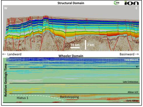
Presenter's notes: By using all of these events for flattening we can create a Wheeler diagram. The Wheeler diagram allows us to visualize a number of things. In this case study the whole interval was divided into 9 stratal packages based on stacking patterns and shifts in depo-centers.
