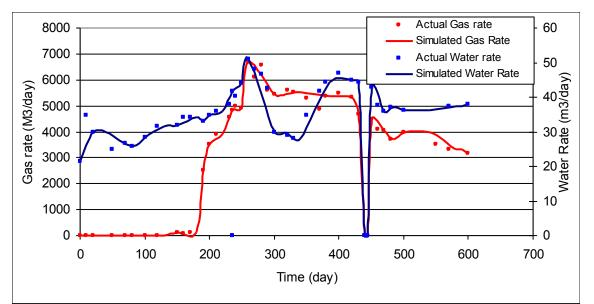
Match the production by adjusting the shrinkage factor and compressibility and initial permeability
