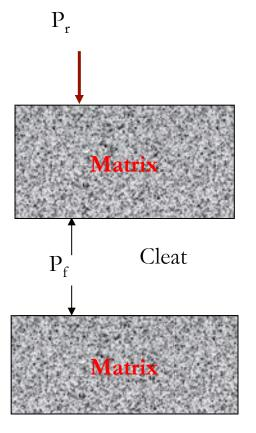
P<sub>r</sub>: pressure caused by load of overlaid rock
