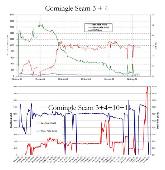
Below Seam 11, there a limestone aquifer Up left: perforated only upper seam, with higher production Low Left: Perforated all seams, low gas and higher water
