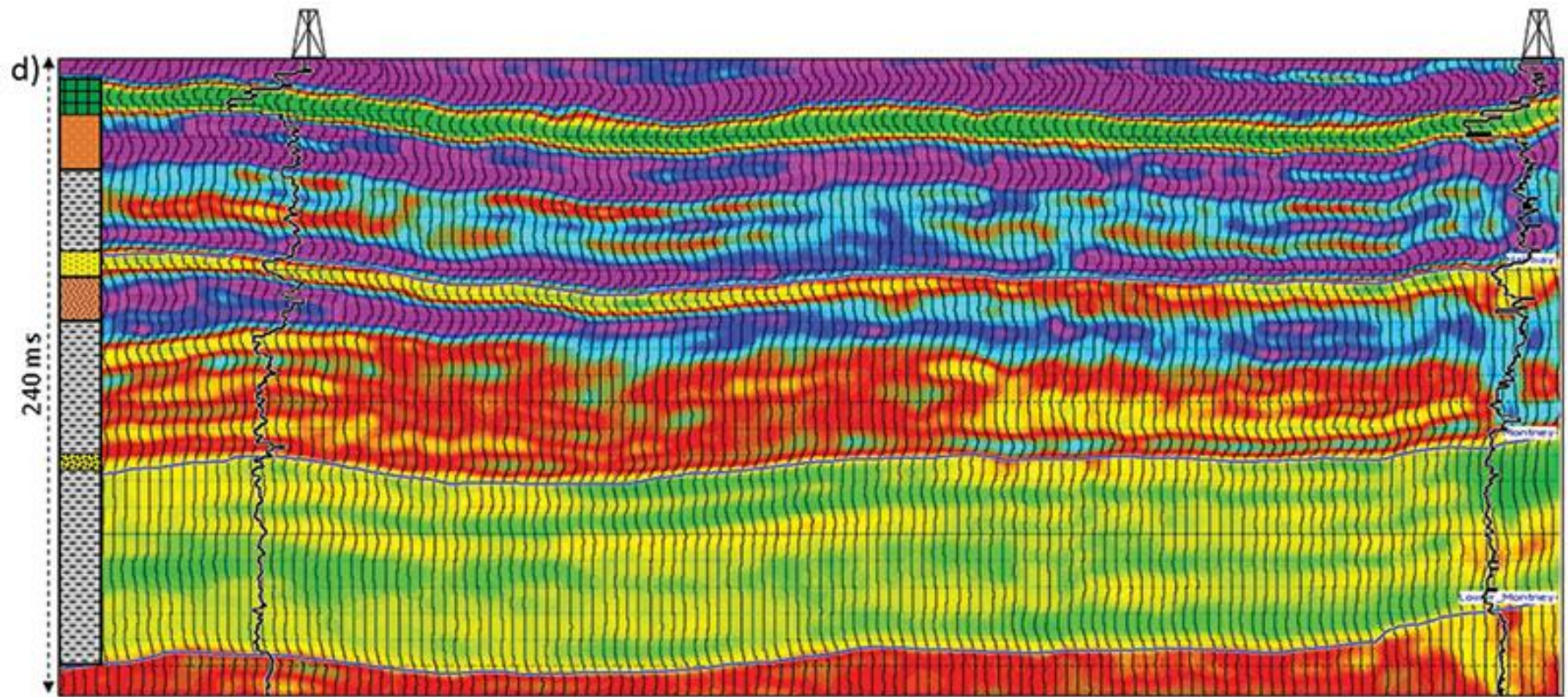
Figure 1d. We show the model-based impedance inversion display. We notice that the impedance variation in the Montney interval appears more detailed than the recursive or colored displays.
