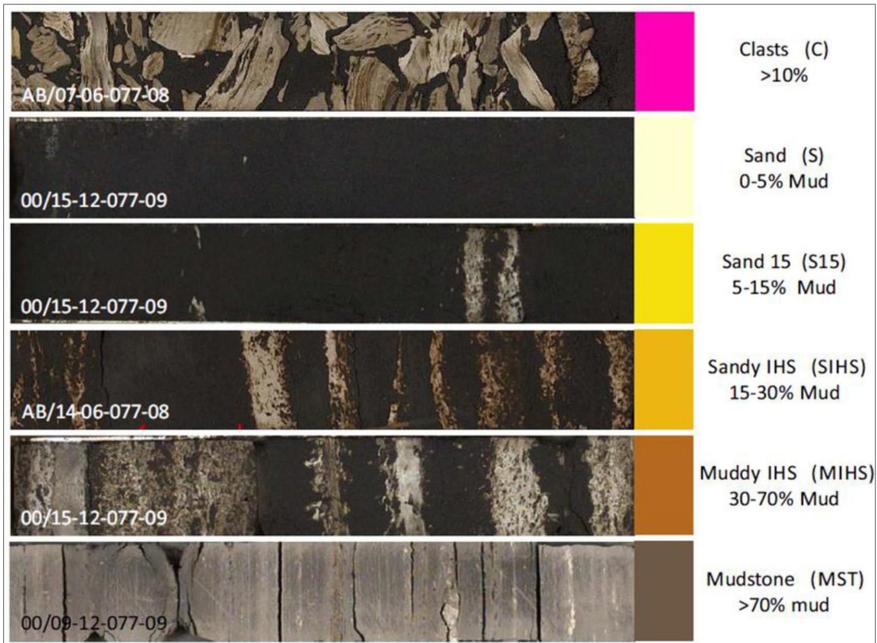
Figure 3. Core examples of the McMurray B lithofacies used in the May River geologic model.
