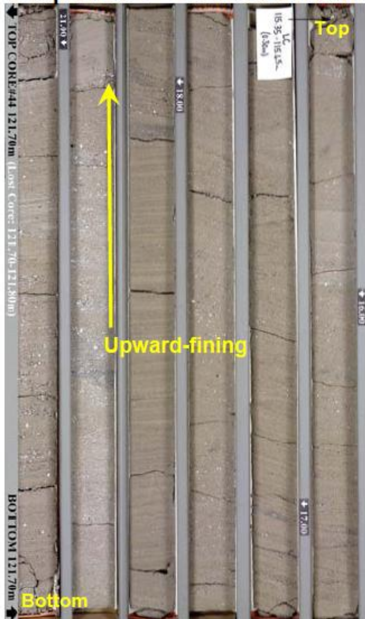
Figure 5. a) Sequence I - Well 06-28-96-07. Water-bearing braided stream sands with trough cross beds and upward-fining beds and bedsets. b) Sequence II - Well 06-29-96-07. Bitumen bearing braided stream sands overlain by finely laminated coastal plain muds.
