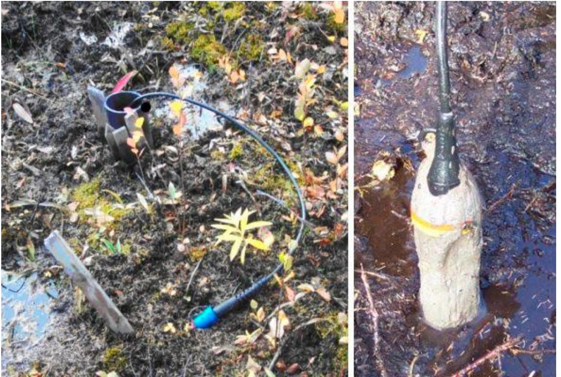
Figure 2. Deployment borehole for a subsurface receiver (left). Retrieved receiver seven months later, showing deployment in clay-mud in subsurface below muskeg (right).
