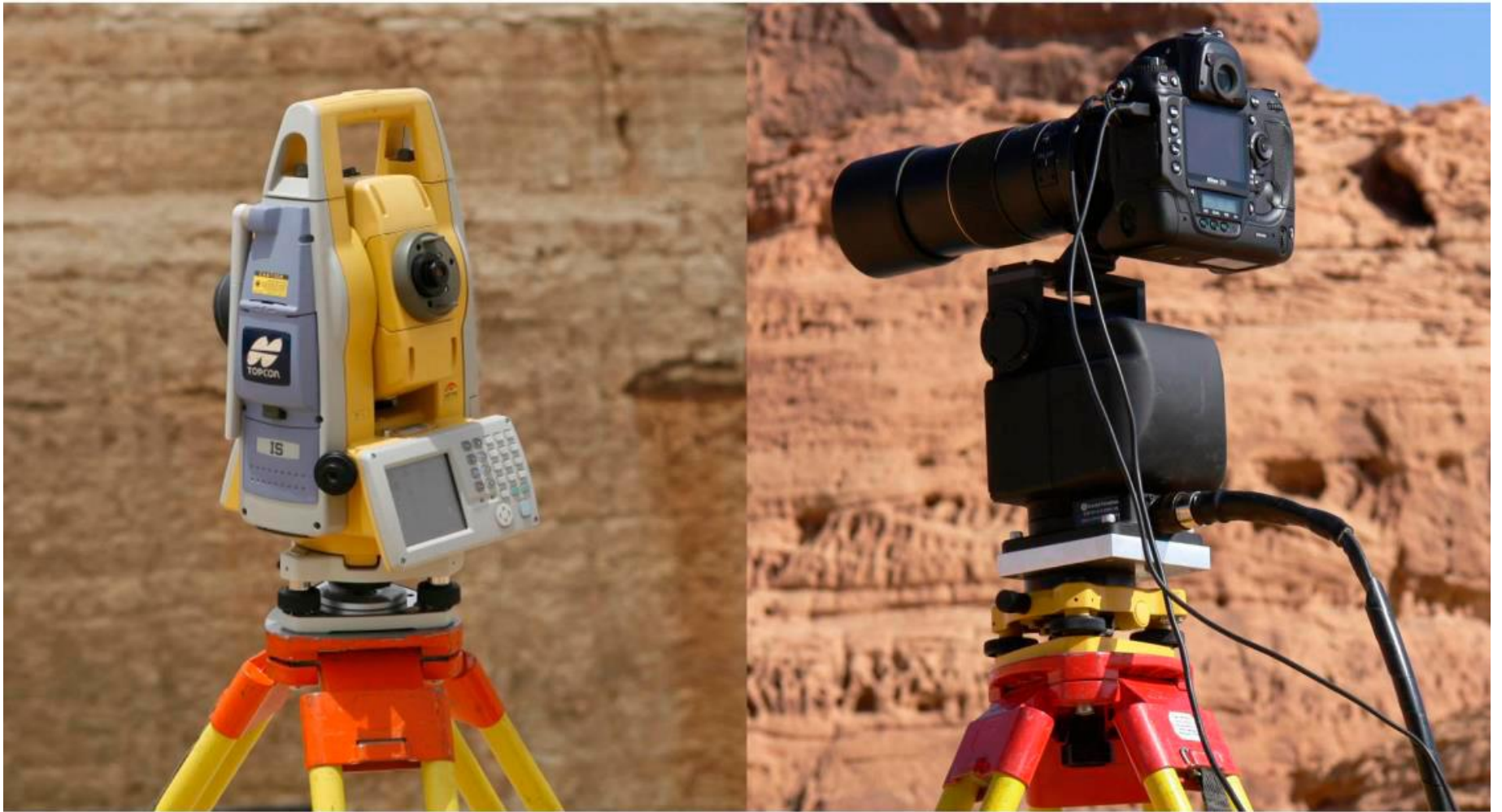
Figure 2. Topcon IS robotic total station on the left. FLIR pan-tilt robot with Nikon D3X DSL camera and 300 mm lens on the right.
