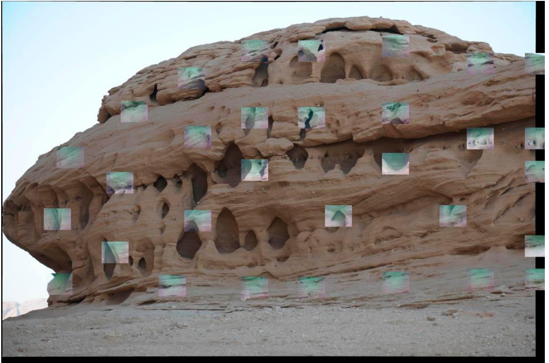
Figure 3. Camera photograph of outcrop with total station cross-hair images superimposed in their approximately correct location.
