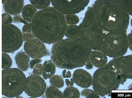
Oolitic grainstone with aggregates. Intergranular porosity (25 - 30%). Presence of open subvertical fractures stained with oil.
