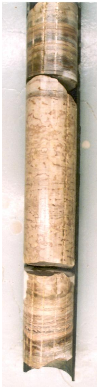
Figure 5. Core photo of an individual cycle from the Midale Evaporite. Note the laminated muds and rooted and burrowed strata (laminated anhydrites not deposited/ preserved here). Cycle averages 1 meter in thickness (7-5-5-4W2M Steelman core).
