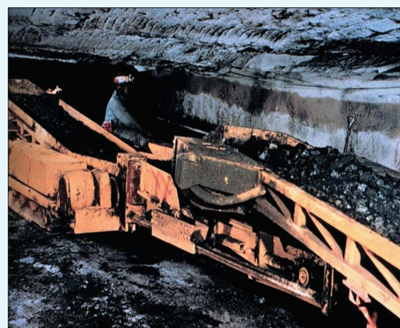
Longwall mining method to extract coal underground in flat-lying strata; "gob" is the coal and surrounding strata above the coal that has collapsed during mining; "gob gas" is a diluted form of CBM emitted from the coal and surrounding strata above the coal during longwall mining owing to seepage of mine air into the gob area; heating values range from 300 to 800 Btu/cf (Bibler and others, 1997; photo courtesy of the Pennsylvania Coal Association).
