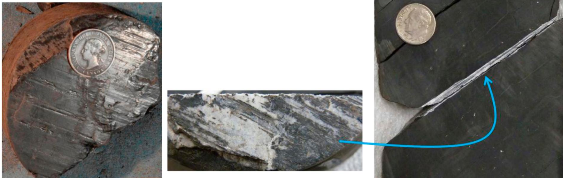
Figure 4. Left, bedding-parallel slip surface in Second White Specks Fm. in Foothills margin region. Right, calcite-lined shear zone and slip surface in dipping beds on flank of large detachment zone, Longmaxi Fm.
