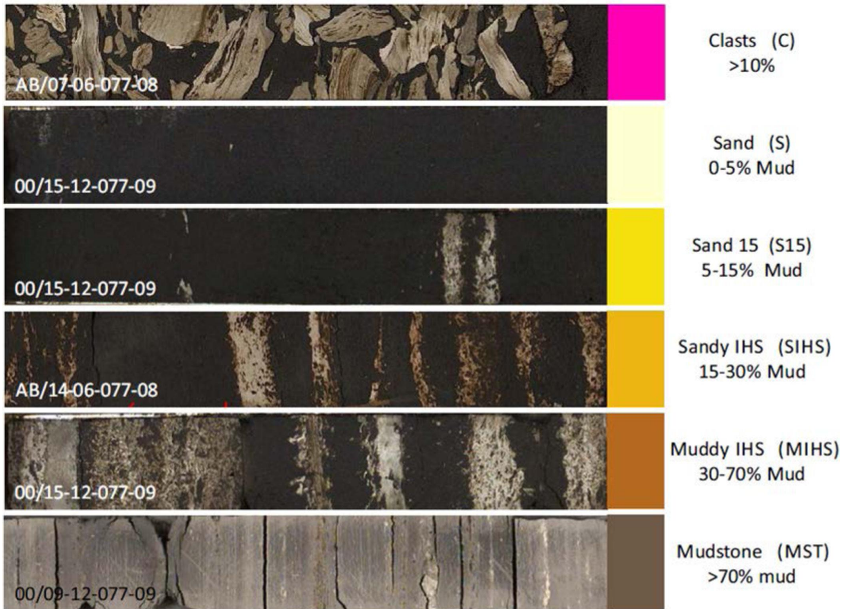
Figure 3. Core examples of the McMurray B lithofacies used in the May River geologic model.
