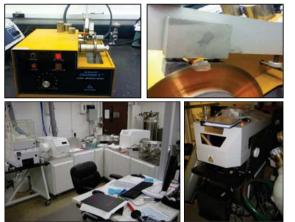
Individual quartz grains are cut along the c-axis using a low speed saw. Silicon isotopic compositions are measured directly on the polished surface of quartz grains using LA-MC-ICP-Ms at University of Houston. Results are reported by δ notation:
