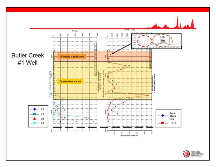
Presenter's notes: The next section is the Queenston and is a very huge section of about a 1,000 ft. The various Strat columns talk about the Queenston as both a sand and a shale indicating the lithology probably varies from clays to sands. The cutting descriptions tend to support that and actually divide this section into an upper and lower section as seen in the next slide.
