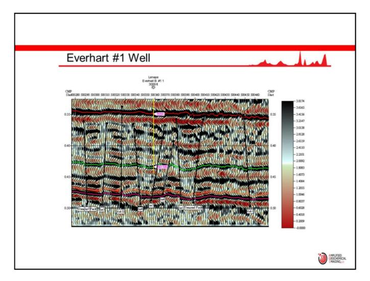
Presenter's notes: Three wells were drilled prior to the Everhart well and each well was noneconomic. This shows basement propagating faults with the Everhart well. The Everhart well was completed in the Trenton formation and was a highly successful well. The IP was approximately 10 mm and then leveled off to 3 mm. This well was used for calibration purposes during the survey because of its high production.
