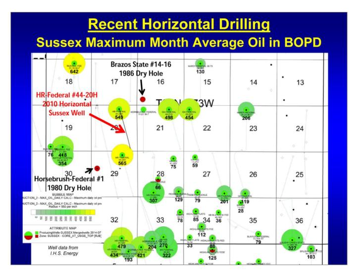
Presenter's notes: Recent horizontal wells have fared much better than the Blaylock, with peak 30-day rates in the 300 to 650 BOPD range. Note that the two dry holes shown on the earlier cross section are now offset by high-volume horizontal producers. An example of a 2010 horizontal Sussex well, the HR-Federal #44-20H, is highlighted with a red arrow and will be shown on the next slide.
