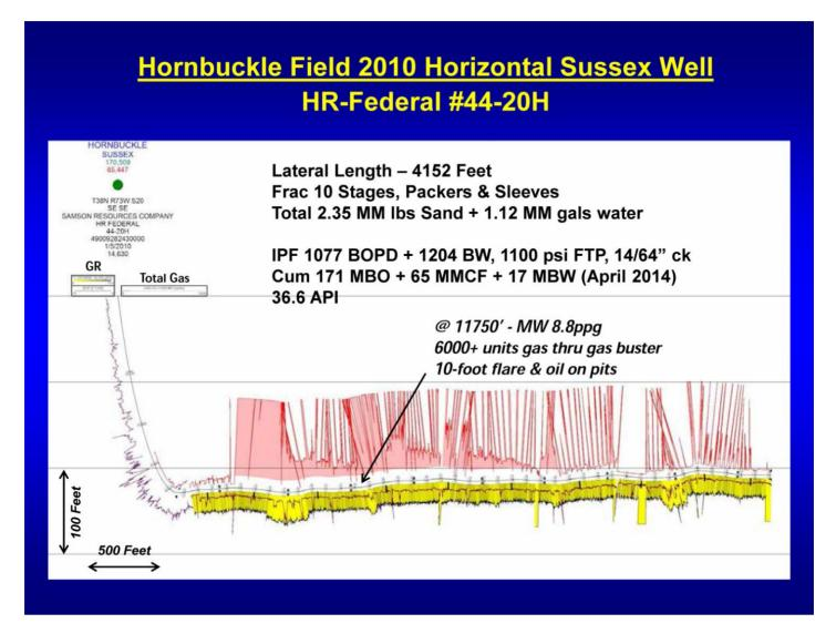
Presenter's notes: A 2010 horizontal Sussex well, the HR-Federal #44-20H. Based on gamma character, most of this lateral was drilled in the bioturbated sandstone facies with only small sections drilled in the cleaner-gamma cross-bedded sandstone facies. This well was completed with a 10-stage fracture stimulation and had a 24-hour IP of 1077 BOPD.
