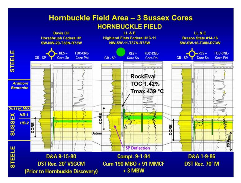
Presenter's notes: Three-well cross section showing three cored wells: a Hornbuckle Field vertical oil producer and two vertical dry holes, both of which are now offset by high-volume horizontal oil producing wells. Logs shown are gamma ray (black) and SP (purple) in track 1, resistivity & core oil saturations in track 2, (*Presenter's notes continued on next slide*)
