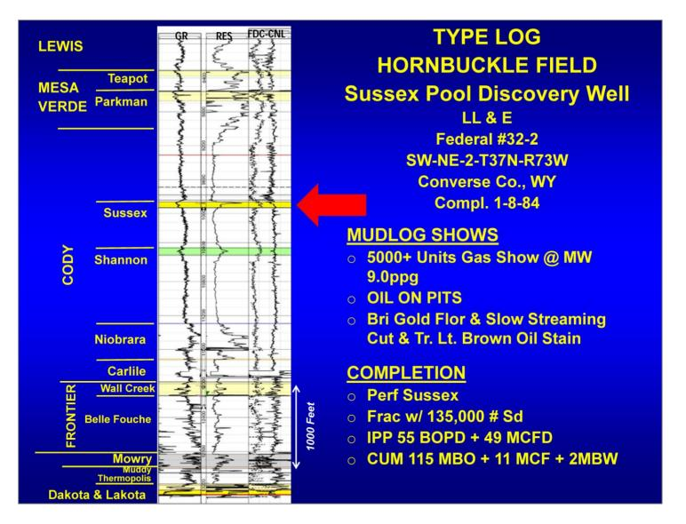
Presenter's notes: Type Log for Hornbuckle Field, showing discovery well drilled by LL&E in 1984. Note excellent show in Sussex while drilling to Muddy-Dakota targets. Hornbuckle was discovered by accident; the prospect was drilled for a deeper objective. Spearhead Ranch/Powell Sussex production was also discovered while drilling for deeper targets.
