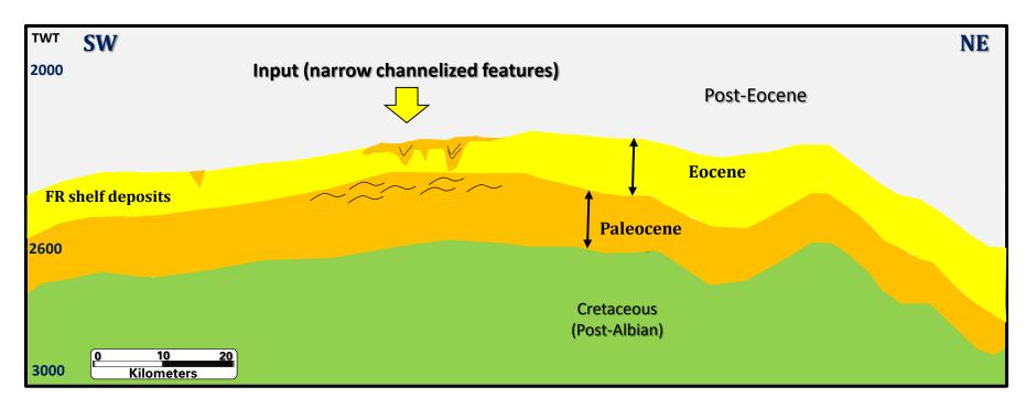
Similar to the Paleocene, the input for Eocene sands is not easy to recognize in the data. It may be here, represented by much narrower channels when compared to the Paleocene section. Again, sparse 2D data is a limitation (Seismic Line 2).
