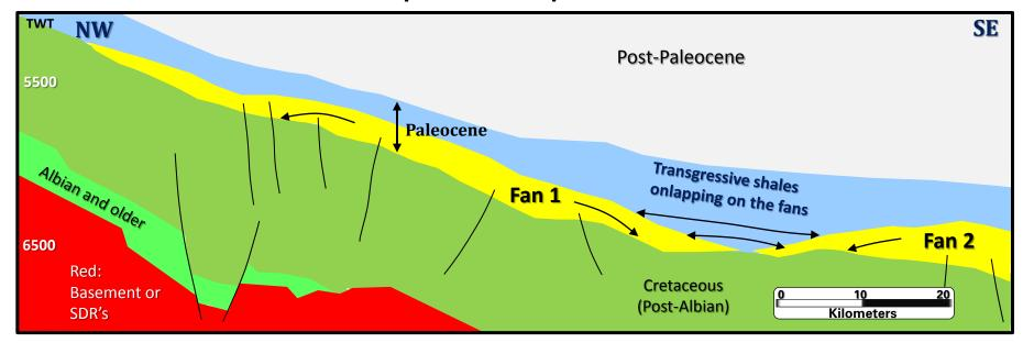
Amalgamation and/or compensation of multiple fans are possible with onlap of the transgressive shales over the lobate geometries.
