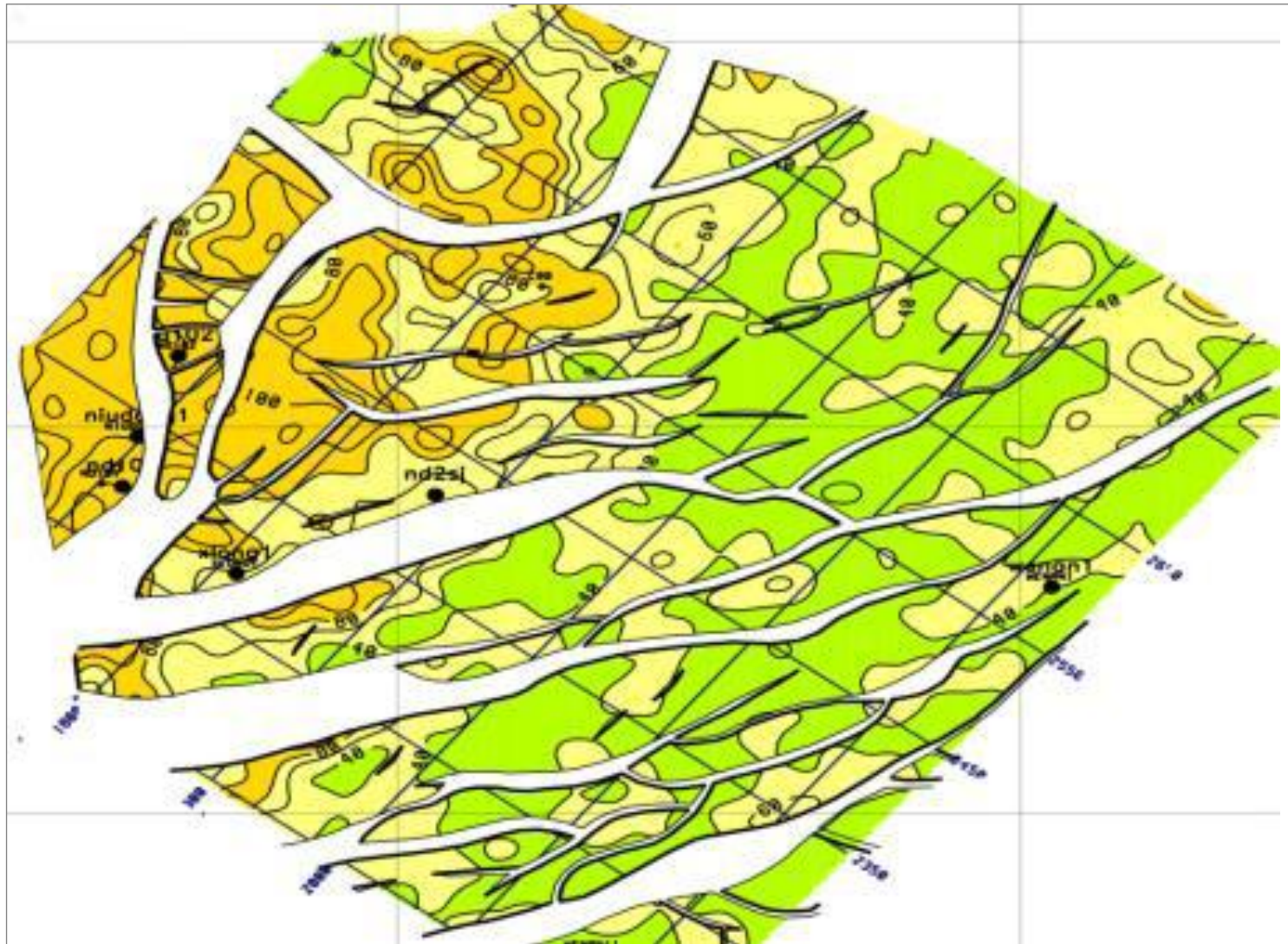
Figure 4. Depth map of hydrocarbon-bearing strata by prestack inversion.
